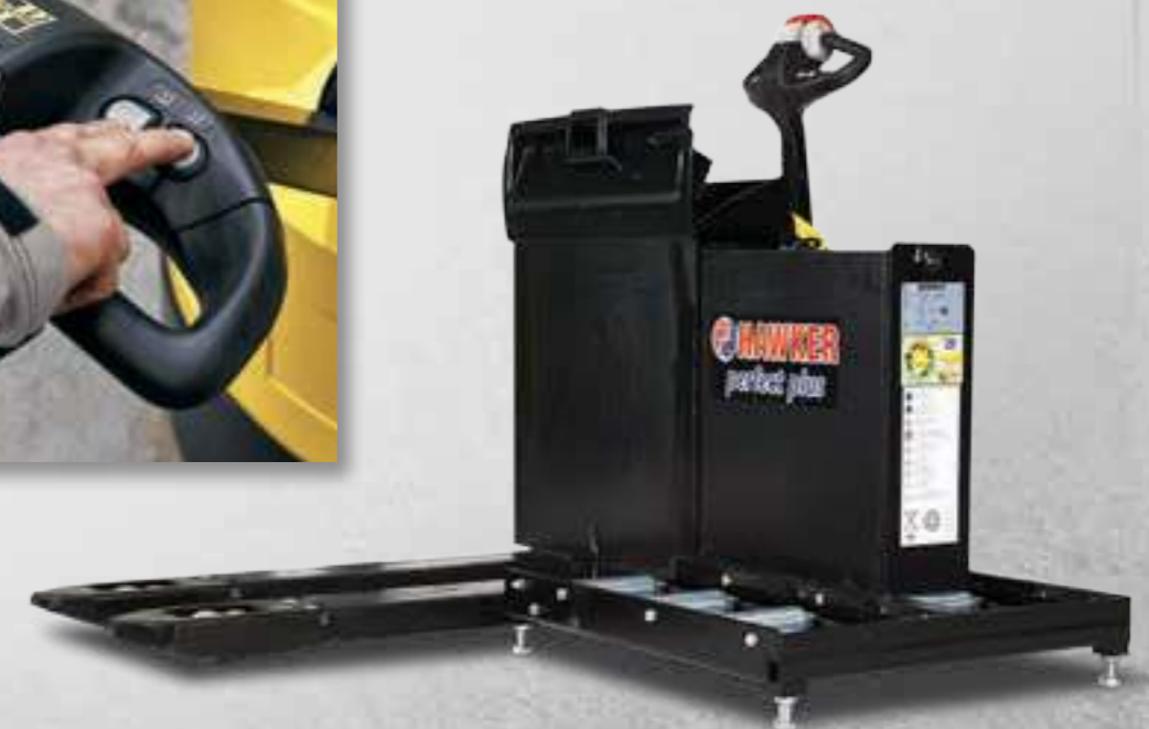
Optional lateral battery extraction system available on P1.8-2.2 models
